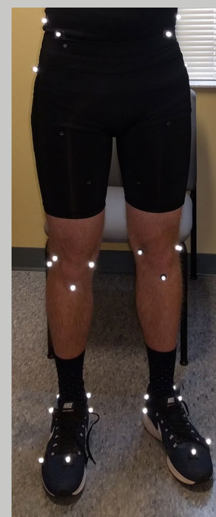
Figure 2: Marker setup used for 3D motion capture.
